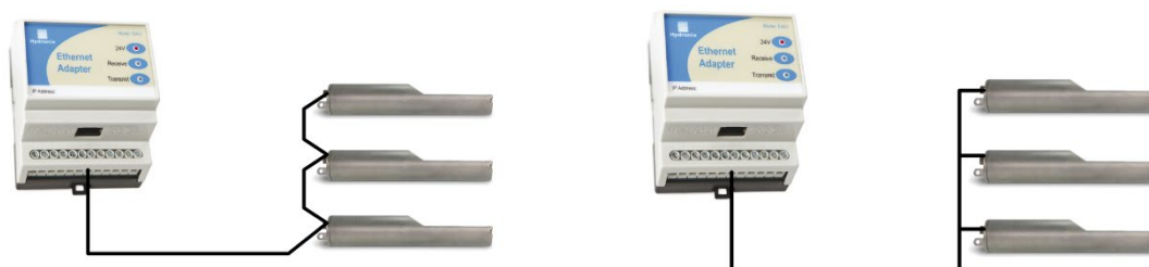
Figure 22: Correct RS485 cable networks
